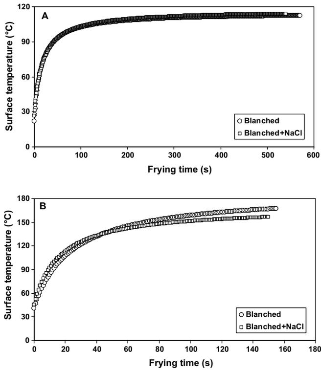
Fig. 1. Surface temperature of control and NaCl soaked potato slices during frying at 120 °C (A) and 180 °C (B).
