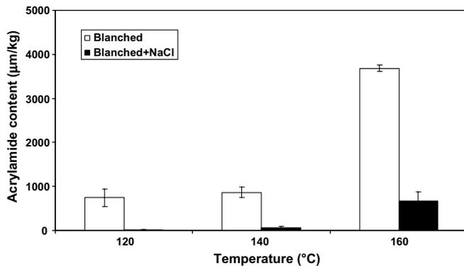
Fig. 5. Acrylamide content for control and NaCl soaked potato chips fried at 120, 140 and 160 °C.
