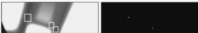
Figure 7. Detection using Method 3: only two of three existing flaws were detected successfully
