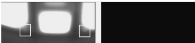
Figure 5. Detection using Method 2: the existing two flaws were not detected
