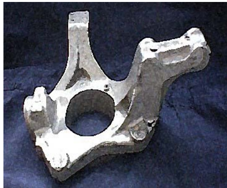
Figure 1: Aluminium casting used in the experiments: a knuckle [Jaeger99].
