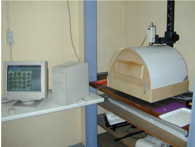
Figure 22.15 Device for quality evaluation of French fries (Gembloux Agricultural University in Belgium).
